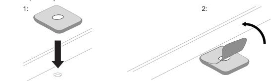
Install the track using M6 T-Bolts, 1/4x3/4mm Flat Washers and M6 Nyloc Nut through each hole in the Track. Place a Plastic Tip over the exposed length of the T-Bolt.
