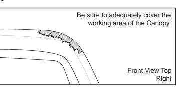
Position the track on the canopy roof so that it fits evenly, illustrated. The aluminium track should be spaced 190mm from the front of the canopy, Use a level or straight edge to locate the very front. Measure 100mm up from the top of the window frame to find the correct position on the apex of the canopy for the tracks. Using a marker, create lines on the masking tape so the track can be easily realigned if it moves.
