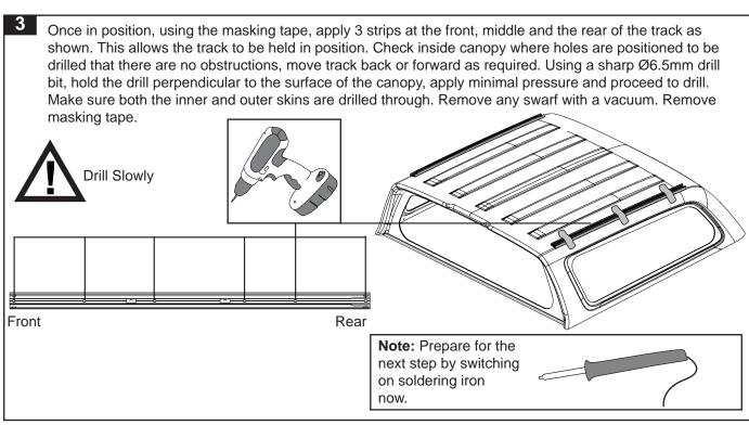
Using a soldering iron, slowly run the hot tip around the circumference of the drilled hole three time. This will seal the ABS from any microcracks that may be present after drilling.
