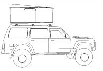
When these roof racks are to be used on a vehicle that is driven off sealed roads the maximum load rating must be divided by 1.5. Remember to subtract the weight of the roof racks to determine your maximum permissible load capacity.
