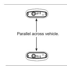
When crossbars are not in use, install the mount cover plates as shown.
