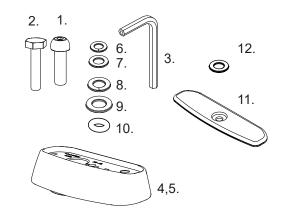
**Tool Required:** Allen Key (provided). Phillips Head Screwdriver. Torx T27 Key.
