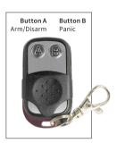
WiTi incorporates an advanced safety system to ensure the system cannot be accidentally activated whilst the caravan or trailer is being towed. After activating the system, if movement is detected during the 3 second safety pause the system will not arm. The lights will not flash twice and the Alarm Status LED will not illuminate.
